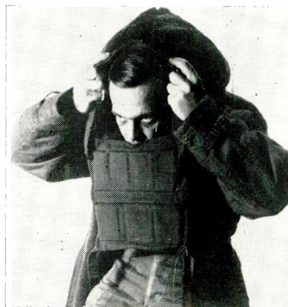
Battery vest is worn under a parka so that body heat will keep the chill out of the cells.
